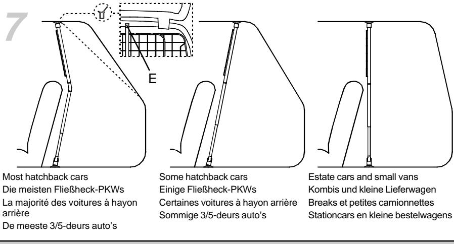
**(GB)** For some hatchback cars, especially those with steeply angled tailgates the top moulding (E) should be used when the tilt foot is unable to provide a secure fit. With the tailgate open, fit the longer side of the top moulding into the gap between the roof and tailgate.
